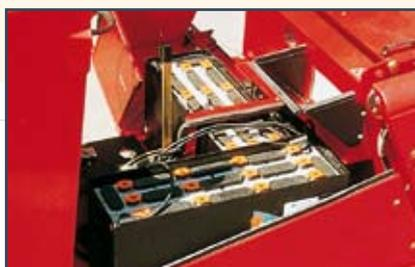
**BATTERY VERSION** Powered at 48V to ensure power and endurance and with hydrostatic transmission for maximum reliability.
