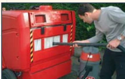
**FILTER CLEANING** The filter can be cleaned without being removed, quickly and without getting dirty, due to a simple vacuum cleaner and the special tube provided.
