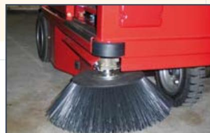
**STRONG** The steel reinforced chassis and the side retractable brushes protect the machine from accidental impacts.
