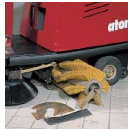
Replacing the main brush is simple and fast.
