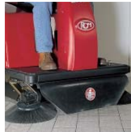
Front dust conveyor to control dust raised by side brushes.
