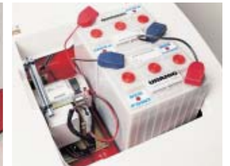
Brava 600 and 700: the two batteries 6V-240Ah.
