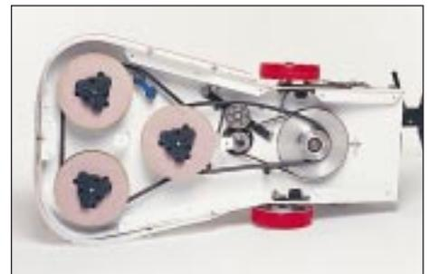
▲ *Easy access to belt and drive system* offers ease of maintenance and serviceability, eliminating costly and unnecessary downtime.
