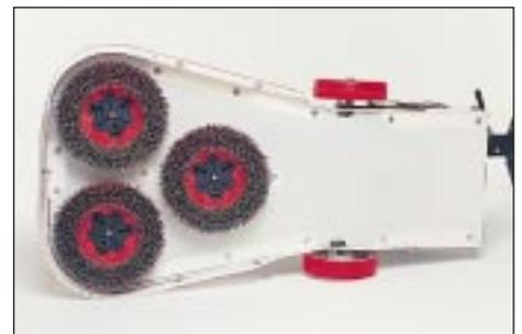
▲ *Pulleys and belts are protected* from contamination by the full underneath splash guard. Fitting and removal of the three Tynex abrasive brushes is quickly and easily facilitated by use of the quick release system.
