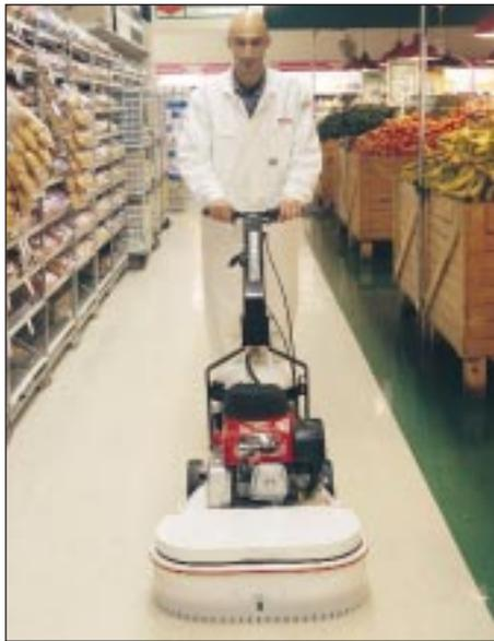
▲ *This versatile stripping machine*, with its removable weight system, can be used for other applications including floor cut back and concrete floor scrubbing.
