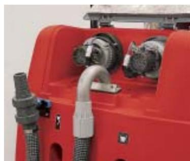
Double vacuum motor to dry perfectly also loose floor or with worn out squeegee
