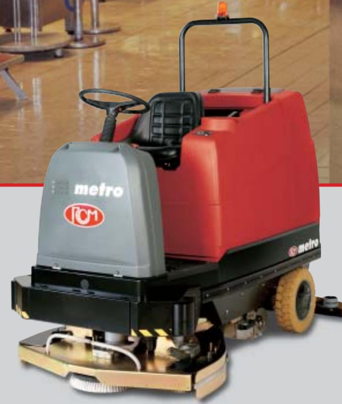
**metro 1103** is a scrubber/drier for large areas. It is powered by a 36 V battery and with a cleaning width of 1070 mm. Strong and simple with easy maintenance, the large diameter wheels give excellent traction on slippery surfaces and slopes. Coupled with the low centre of gravity by placing the large traction battery low in the chassis gives the **metro 1103** stability and comfort.
