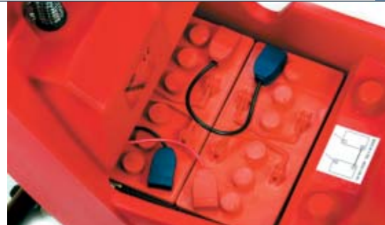
The battery housing (532) contains lead or gel batteries up to 140A (20h), this means GO can work for more than 4 hours.
